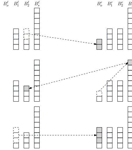
Fig. 3: An example of how funds are transferred across a payment channel and how buckets are refilled. Both \ell and r start with full buckets. The first transaction is in the left-to-right direction and is transferred using funds from B_2^l to B_0^r . The second transaction is in the right-to-left direction and is small, thus funds from B_s^r are used. B_s^r is immediately refilled using funds from B_0^r . The third transaction is in the left-to-right direction and uses funds from B_1^l .
